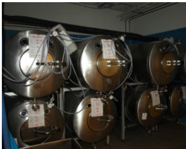
Figure 8.73 Fermentation of grape juice to make wine produces \text{CO}_2 as a byproduct. Fermentation tanks have valves so that pressure inside the tanks can be released.
